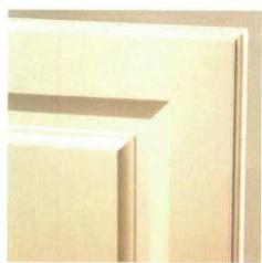
Thermofoil doors have a core of engineered wood. A traditional frame-and-panel look-alike, this door is actually a vinyl-like plastic formed around a core of medium-density fiberboard milled by a computer-controlled router. Unlike other kinds of laminated doors, this one has only a single seam. MDF is heavy and stable.
